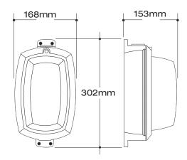
FIXING POINTS: 4 X 8mm dia. holes on 280 x 32mm centres
