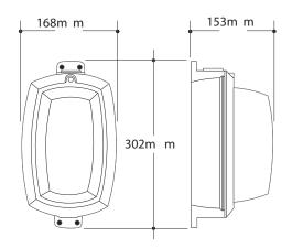
FIXING POINTS: 4 X 8mm dia. holes on 280 x 32mm centre
