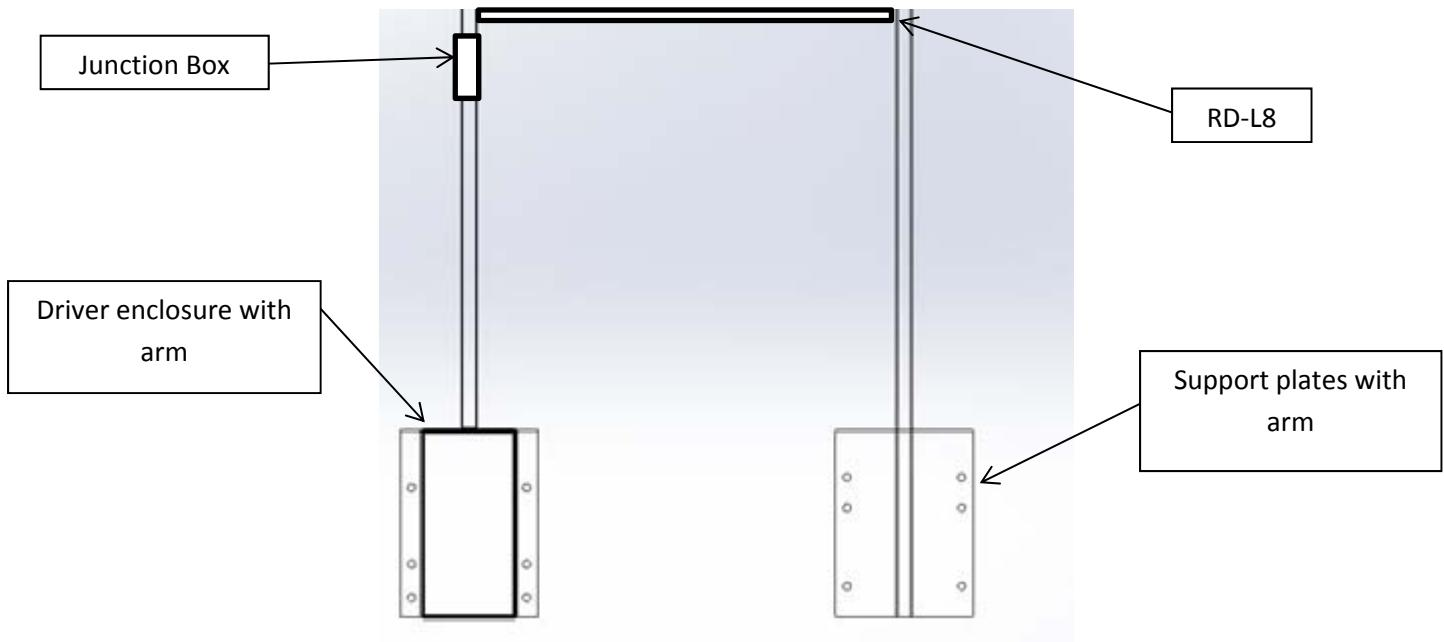
1. Insert the RD-L8 into the first arm, ensure the fixture wire side is oriented towards the driver box arm, and not towards the support arm. Wire the fixture using the quick connects. Once the fixture is connected, test the fixture to ensure proper function. Troubleshoot connections as necessary. See image below for mounting details.
