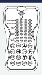
BRIGHTNESS: Sets the highest light fixture brightness when motion is detected.
