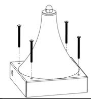
4. Remove the reflector mount plate by removing the four corner screws as shown in figure to access branch connections.
