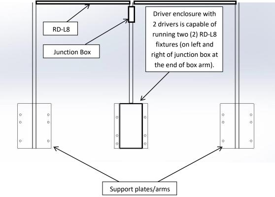
3. Insert the first RD-L8 into the first arm, ensure the fixture wire side is oriented towards the driver box arm, and not the support arm. Wire the fixtures using the quick connects. Once all fixtures are connected, test the fixture to ensure proper function. Troubleshoot connections as necessary. See image below for mounting details.
