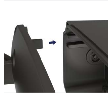
Fixture head has guide tabs that slide into the channel and lock it in place. goes into keyholes allowing installer to use both hands for wiring.
