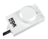
The High Frequency Motion Sensor uses high frequency waves to detect motion. The sensor sends out waves that bounce off nearby surfaces and return to the sensor. Motion changes the speed of the waves returning to the sensor. The sensor detects the change in speed and interprets it as occupancy which causes the light to turn on. It triggers primarily through movement of people, objects, machinery. The band of frequency that it usually operates in is <10 mW (about 10x lower than mobile phones)
