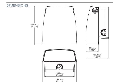
The AWL-LED14W is a multi-purpose fixture that can be used to replace wall packs and floods up to 150 watt metal halide.The head can be aimed straight down for dark sky requirements or aimed out to deliver the light where it is required.
